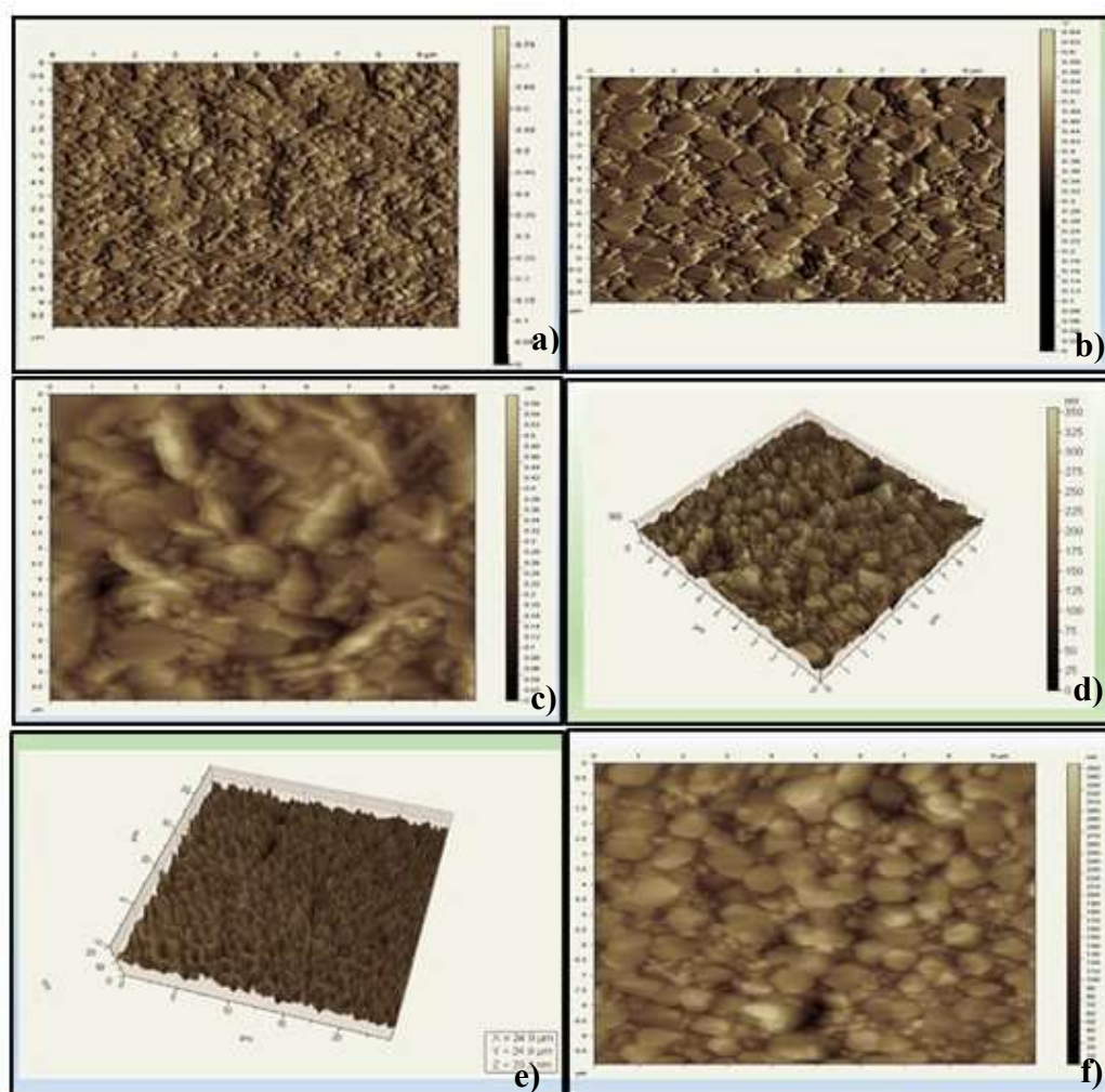
Fig. 4. Morphology obtained by AFM of thin films spin coated for 30 s (a and b), 40 s (c and d) and 50 s (e and f).
