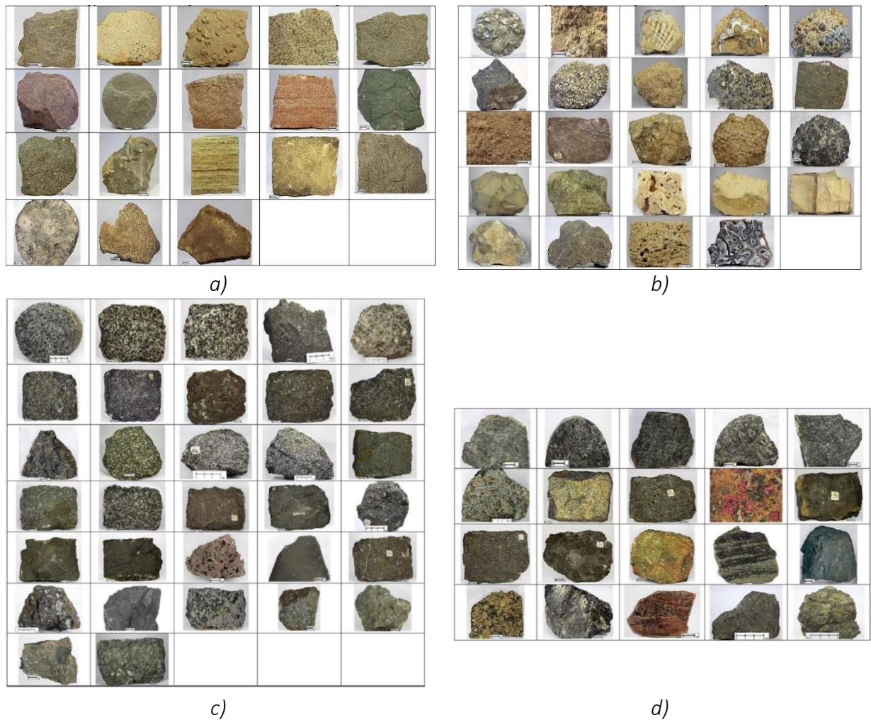
Fig. 2. Photographs of rock samples whose resonant frequencies are used during images processing: a) 2nd group of sedimentary rocks (psammities); b) 7th group of sedimentary rocks (limestones); c) 6th group igneous rocks (gabbros and basalts); d) group 7 igneous (ultramafic) rocks.
