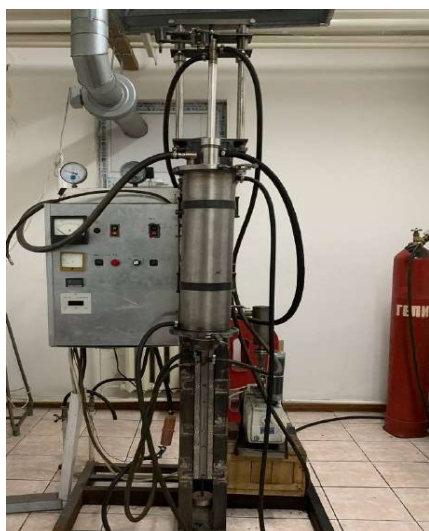
Fig.1-plant for the production of fullerenes in a helium medium
