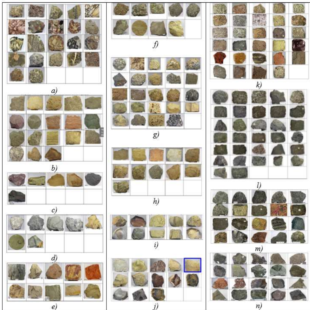
Fig. 3. Photographs of rock samples whose resonant frequencies are used during images processing [3]: a) psephites, monomineralic conglomerates; b) psammites; c) silts, mudstones, clays; d) kaolinite mudstones; e) kaolinite clays; f) sedimentary-volcaniclastic rocks; tuff breccias; g) limestones; h) dolomites; i) marls; j) siliceous rocks; k) 1st group of granite rocks; l) gabbros and basalts; m) 7th group of igneous (ultramafic) rocks; n) kimberlites and lamproites.
