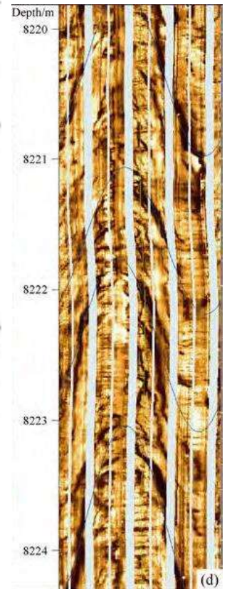
Fig. 8. Lithology and FMI characteristics of the reservoir in the Sinian Qigebulake Formation and the Lower Cambrian Wusonggeer Formation; (d) fractures and dissolved cavities [30].
