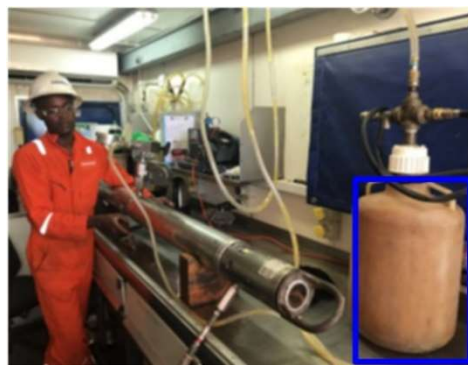
Fig. 22. Blowdown of Pebbly Arkose fluid sample where natural gas was recovered from a depth of 2197.3mMD [4].
