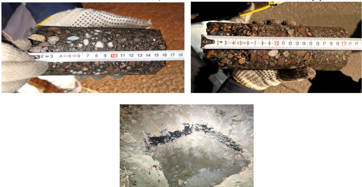
Fig. 1 – drilled core from asphalt concrete pavement
