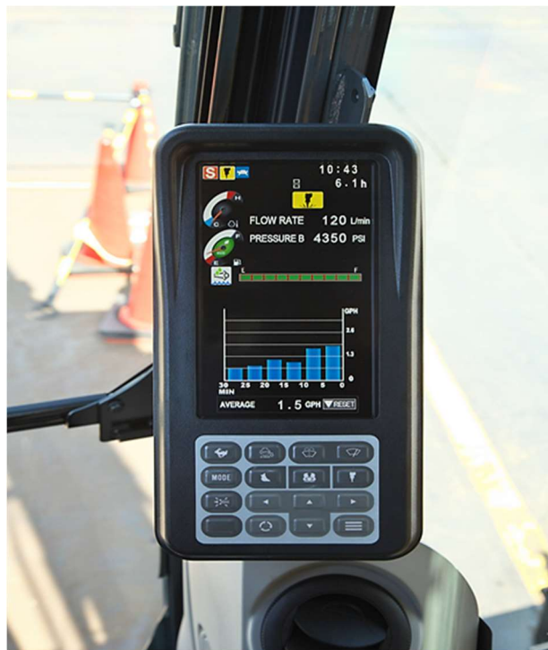
Figure 1. Excavator on-board diagnostic display showing real-time performance metrics.
