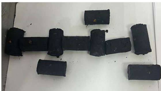
Figure 1 – Briquettes made from Sarykol coal and food waste
