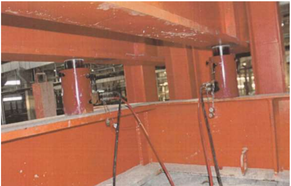
Figure 2.18 - Loading system with hydraulic jacks
