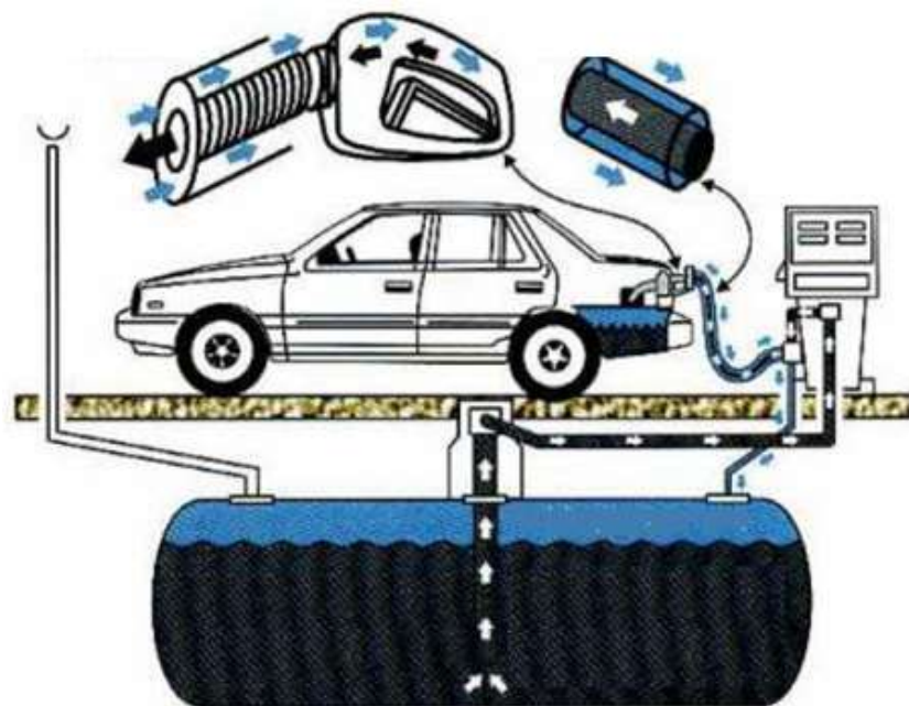
Figure 4-Gas balancing system for bypassing vapors when refueling a car: blue area-gasoline vapors; gray area-gasoline
