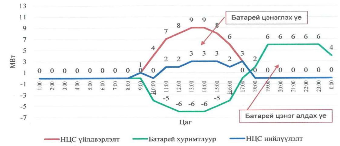
Figure 4. Scheme of the combined operation of a solar power plant with a capacity of 10 MW and batteries.
