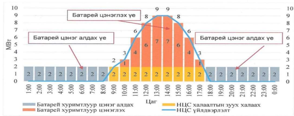
Figure 5. Schematic diagram of the combined operation of a solar power plant and batteries.
