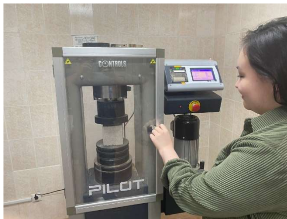
Figure 3. Testing of a sample of non-autoclaved aerated concrete without fiber for strength
