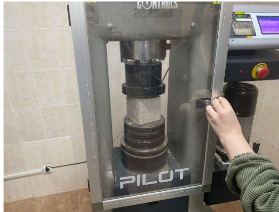
Figure 3. Testing of a sample of non-autoclaved aerated concrete without fiber for strength
