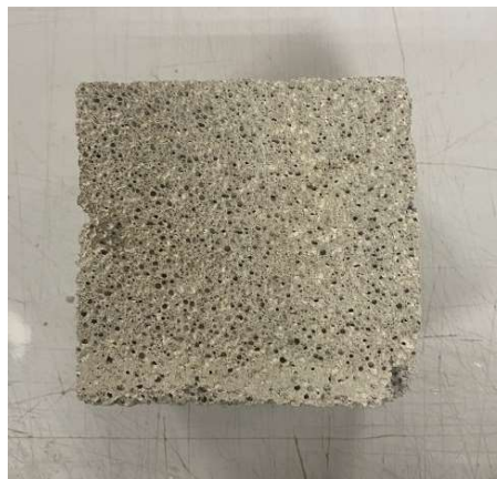
Fig.6 Sample of non-autoclaved aerated concrete with fiber after strength testing
