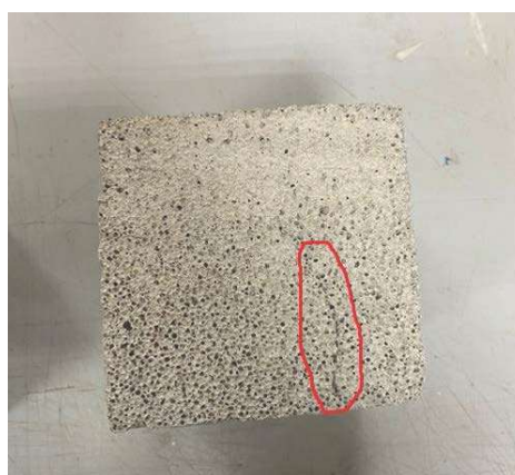
Fig.5 Sample of non-autoclaved aerated concrete without fiber after strength testing
