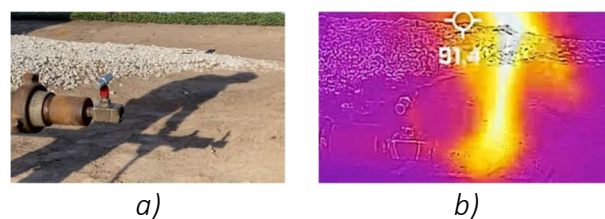
Fig. 10. Foto images B of a transparent flame in normal light (a) and the flame in infrared camera [9].
