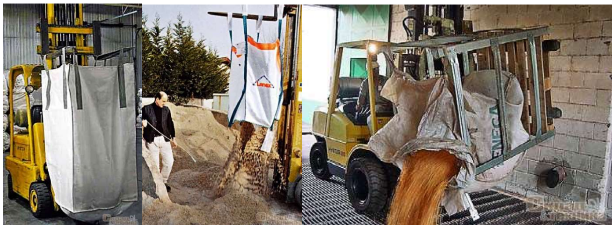
Pic. 2.1 – Example of using the soft cone forks.
