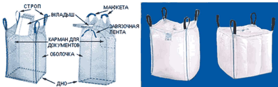
Pic. 1.5 – soft container “Big Bag”: a.– external view, b) – constructional elements
