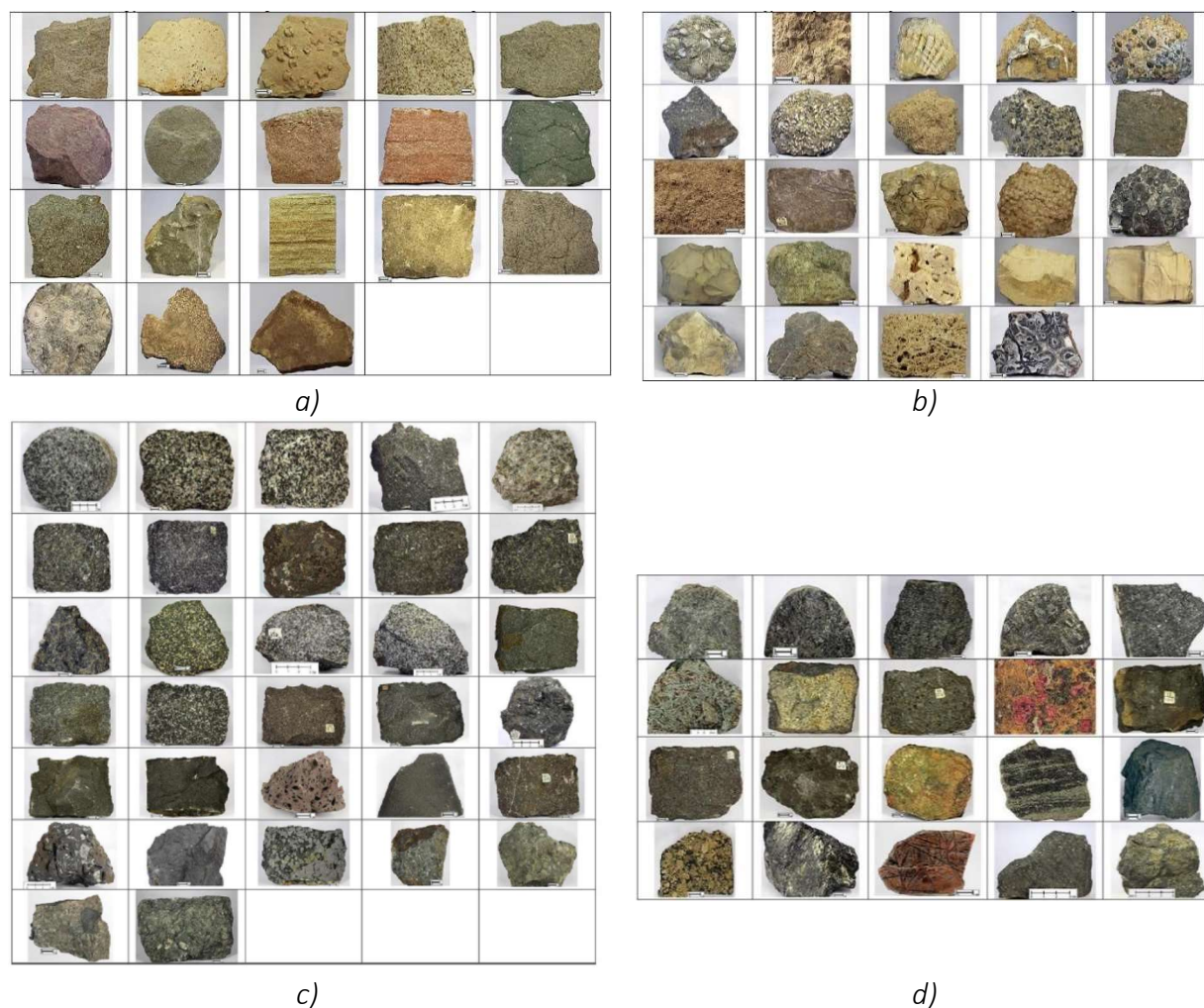
Fig. 2. Photographs of rock samples whose resonant frequencies are used during images processing: a) 2nd group of sedimentary rocks (psammites); b) 7th group of sedimentary rocks (limestones); c) 6th group igneous rocks (gabbros and basalts); d) group 7 igneous (ultramafic) rocks.
